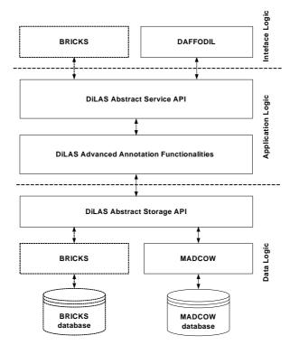
Figure 2 : Architecture of the DiLAS system.
